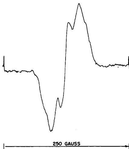
Fig. 5. ESR spectra of cotton cellulose II generated by the \text{Fe}^{+2}/\text{H}_2\text{O}_2 system plus acrylonitrile, recorded at -40^\circ\text{C} . ( \times 2500 ).
